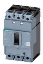
circuit breaker 3VM1 IEC frame 160 breaking capacity class M Icu=55kA @ 415V 3-pole, starter protection TM120M, AM, In=80A without overload protection short-circuit protection Ii=7...16 x In nut keeper kit
