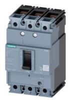
circuit breaker 3VM1 IEC frame 160 breaking capacity class M Icu=55kA @ 415V 3-pole, starter protection TM120M, AM, In=50A without overload protection short-circuit protection Ii=7...16 x In nut keeper kit
