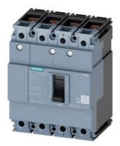
circuit breaker 3VM1 IEC frame 160 breaking capacity class M Icu=55kA @ 415V 4-pole, line protection TM210, FTFM, In=50A overload protection Ir=50A, not adjustable short-circuit protection Ii=10 x In N conductor protection 100% nut keeper kit
