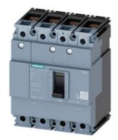
circuit breaker 3VM1 IEC frame 160 breaking capacity class S Icu=36kA @ 415V 4-pole, line protection TM210, FTFM, In=50A overload protection Ir=50A, not adjustable short-circuit protection Ii=10 x In N conductor protection 100% nut keeper kit
