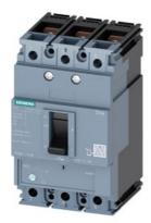
circuit breaker 3VM1 IEC frame 160 breaking capacity class S Icu=36kA @ 415V 3-pole, line protection TM220, ATFM, In=50A overload protection Ir=35A...50A short-circuit protection Ii=10 x In nut keeper kit
