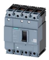
circuit breaker 3VM1 IEC frame 160 breaking capacity class S Icu=36kA @ 415V 4-pole, line protection TM220, ATFM, In=40A overload protection Ir=28A...40A short-circuit protection Ii=10 x In N conductor protection 100% nut keeper kit
