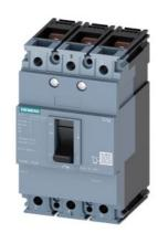
circuit breaker 3VM1 IEC frame 160 breaking capacity class S Icu=36kA @ 415V 3-pole, line protection TM210, FTFM, In=40A overload protection Ir=40A, not adjustable short-circuit protection Ii=10 x In nut keeper kit
