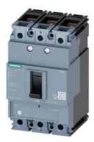
circuit breaker 3VM1 IEC frame 160 breaking capacity class N Icu=25kA @ 415V 3-pole, line protection TM220, ATFM, In=40A overload protection Ir=28A...40A short-circuit protection Ii=10 x In nut keeper kit
