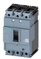
circuit breaker 3VM1 IEC frame 160 breaking capacity class M Icu=55kA @ 415V 3-pole, starter protection TM120M, AM, In=32A without overload protection short-circuit protection Ii=7...16 x In nut keeper kit
