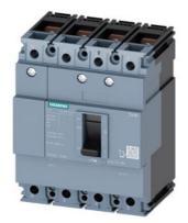
circuit breaker 3VM1 IEC frame 160 breaking capacity class S Icu=36kA @ 415V 4-pole, line protection TM210, FTFM, In=32A overload protection Ir=32A, not adjustable short-circuit protection Ii=10 x In N conductor protection 100% nut keeper kit
