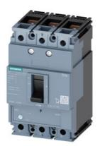
circuit breaker 3VM1 IEC frame 160 breaking capacity class N Icu=25kA @ 415V 3-pole, line protection TM220, ATFM, In=32A overload protection Ir=22A...32A short-circuit protection Ii=10 x In nut keeper kit
