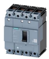
circuit breaker 3VM1 IEC frame 160 breaking capacity class S Icu=36kA @ 415V 4-pole, line protection TM220, ATFM, In=25A overload protection Ir=18A...25A short-circuit protection Ii=12.8 x In N conductor protection 100% nut keeper kit
