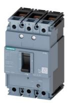
circuit breaker 3VM1 IEC frame 160 breaking capacity class M Icu=55kA @ 415V 3-pole, starter protection TM120M, AM, In=20A without overload protection short-circuit protection Ii=7...16 x In nut keeper kit
