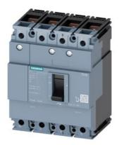
circuit breaker 3VM1 IEC frame 160 breaking capacity class M Icu=55kA @ 415V 4-pole, line protection TM210, FTFM, In=20A overload protection Ir=20A, not adjustable short-circuit protection Ii=16 x In N conductor protection 100% nut keeper kit
