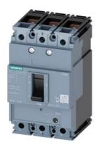
circuit breaker 3VM1 IEC frame 160 breaking capacity class M Icu=55kA @ 415V 3-pole, starter protection TM120M, AM, In=125A without overload protection short-circuit protection li=7...16 x In nut keeper kit
