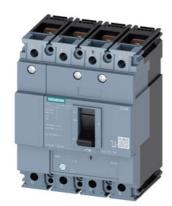
circuit breaker 3VM1 IEC frame 160 breaking capacity class S Icu=36kA @ 415V 4-pole, line protection TM220, ATFM, In=125A overload protection Ir=88A...125A short-circuit protection Ii=10 x In N conductor protection 100% nut keeper kit
