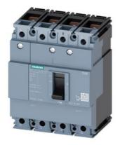
circuit breaker 3VM1 IEC frame 160 breaking capacity class N Icu=25kA @ 415V 4-pole, line protection TM210, FTFM, In=125A overload protection Ir=125A, not adjustable short-circuit protection Ii=10 x In N conductor unprotected nut keeper kit
