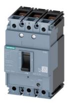
circuit breaker 3VM1 IEC frame 160 breaking capacity class M Icu=55kA @ 415V 3-pole, starter protection TM120M, AM, In=100A without overload protection short-circuit protection li=7...16 x In nut keeper kit
