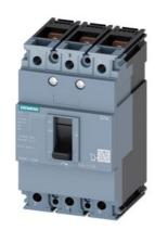
circuit breaker 3VM1 IEC frame 160 breaking capacity class M Icu=55kA @ 415V 3-pole, starter protection TM110M, FM, In=8A without overload protection short-circuit protection Ii=15 x In nut keeper kit
