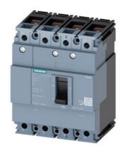
circuit breaker 3VM1 IEC frame 100 breaking capacity class N Icu=25kA @ 415V 4-pole, line protection TM210, FTFM, In=16A overload protection Ir=16A, not adjustable short-circuit protection Ii=20 x In N conductor unprotected nut keeper kit
