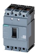
circuit breaker 3VM1 IEC frame 100 breaking capacity class N Icu=25kA @ 415V 3-pole, line protection TM210, FTFM, In=80A overload protection Ir=80A, not adjustable short-circuit protection Ii=10 x In nut keeper kit
