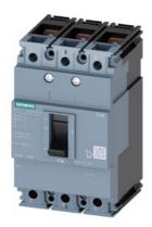
circuit breaker 3VM1 IEC frame 100 breaking capacity class B Icu=16kA @ 415V 3-pole, line protection TM210, FTFM, In=80A overload protection Ir=80A, not adjustable short-circuit protection Ii=10 x In nut keeper kit
