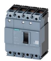
circuit breaker 3VM1 IEC frame 100 breaking capacity class N Icu=25kA @ 415V 4-pole, line protection TM210, FTFM, In=63A overload protection Ir=63A, not adjustable short-circuit protection li=10 x In N conductor unprotected nut keeper kit
