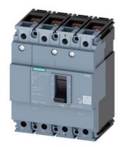
circuit breaker 3VM1 IEC frame 100 breaking capacity class B Icu=16kA @ 415V 4-pole, line protection TM210, FTFM, In=63A overload protection Ir=63A, not adjustable short-circuit protection Ii=10 x In N conductor unprotected nut keeper kit
