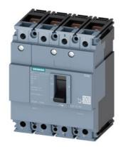
circuit breaker 3VM1 IEC frame 100 breaking capacity class N Icu=25kA @ 415V 4-pole, line protection TM210, FTFM, In=25A overload protection Ir=25A, not adjustable short-circuit protection Ii=12.8 x In N conductor unprotected nut keeper kit
