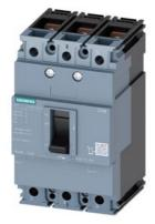
circuit breaker 3VM1 IEC frame 100 breaking capacity class N Icu=25kA @ 415V 3-pole, line protection TM210, FTFM, In=25A overload protection Ir=25A, not adjustable short-circuit protection Ii=12.8 x In nut keeper kit
