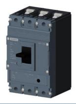
circuit breaker 3VJ1 IEC framesize 3VJ11 125A line protection ATFM 3-pole lcu=36kA@415V lcs=75% lcu In=125A overload protection Ir=100A...125A short-circuit protection Ii=10 x In Screw connection
