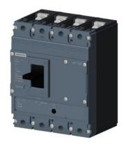
circuit breaker 3VJ1 IEC framesize 3VJ11 125A line protection ATFM 4-pole lcu=55kA@415V lcs=75% lcu ln=100A overload protection lr=80A...100A short-circuit protection li=10 x ln Screw connection
