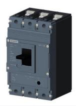
circuit breaker 3VJ1 IEC framesize 3VJ11 125A line protection ATFM 3-pole Icu=55kA@415V Ics=75% Icu In=80A overload protection Ir=64A...80A short-circuit protection Ii=10 x In Screw connection
