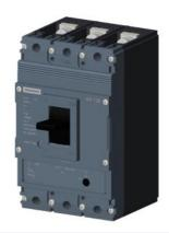
circuit breaker 3VJ1 IEC framesize 3VJ11 125A line protection ATFM 3-pole Icu=36kA@415V Ics=75% Icu In=80A overload protection Ir=64A...80A short-circuit protection Ii=10 x In Screw connection
