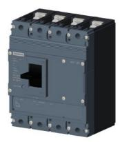
circuit breaker 3VJ1 IEC framesize 3VJ11 125A line protection FTFM 4-pole Icu=36kA@415V Ics=75% Icu In=63A overload protection Ir=63A short-circuit protection Ii=10 x In Screw connection
