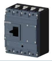
circuit breaker 3VJ1 IEC framesize 3VJ11 125A line protection ATFM 4-pole Icu=55kA@415V Ics=75% Icu In=50A overload protection Ir=40A...50A short-circuit protection Ii=600A Screw connection
