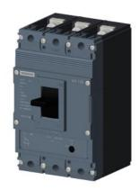
circuit breaker 3VJ1 IEC framesize 3VJ11 125A line protection ATFM 3-pole Icu=55kA@415V Ics=75% Icu In=50A overload protection Ir=40A...50A short-circuit protection Ii=600A Screw connection
