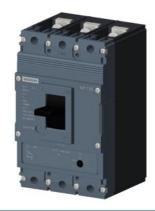
circuit breaker 3VJ1 IEC framesize 3VJ11 125A line protection ATFM 3-pole Icu=36kA@415V Ics=75% Icu In=50A overload protection Ir=40A...50A short-circuit protection Ii=600A Screw connection
