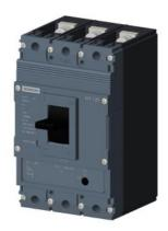
circuit breaker 3VJ1 IEC framesize 3VJ11 125A line protection ATFM 3-pole Icu=55kA@415V Ics=75% Icu In=40A overload protection Ir=32A...40A short-circuit protection Ii=600A Screw connection
