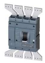
circuit breaker 3VA2 IEC Frame 1250 breaking capacity class M Icu=55 kA @ 415 V 4-pole, line protection ETU330, LIG, In=1250 A overload protection Ir=500 A ...1250 A short-circuit protection Ii=1.5...10 x In neutral conductor protection adjustable (OFF, 50%, 100%) ground-fault protection Ig=0.2... 1 x In, tg=0.1/0.3s bus connectors broadened
