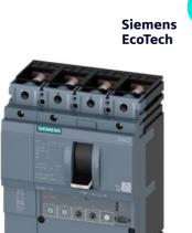
circuit breaker 3VA2 IEC Frame 100 breaking capacity class S Icu=36 kA @ 415 V 4-pole, line protection ETU330, LIG, In=40 A overload protection Ir=16 A...40 A short-circuit protection Ii=1.5...12 x In neutral conductor protection adjustable (OFF, 100%) ground-fault protection Ig=0.4...1 x In= tg=0.1/0.3s nut keeper kit
