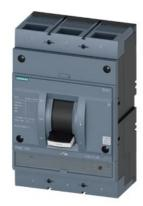
circuit breaker 3VA1 IEC Frame 1000 breaking capacity class M Icu=55 kA @ 415 V 3-pole, starter protection TM120M, AM, In=800 A without overload protection short-circuit protection Ii=6...12 x In nut keeper kit
