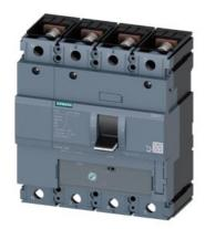
circuit breaker 3VA1 IEC Frame 250 breaking capacity class M Icu=55 kA @ 415 V 4-pole, line protection TM220, ATFM, In=250 A overload protection Ir=175 A...250 A short-circuit protection Ii=10 x In neutral conductor protection 100% nut keeper kit
