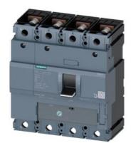
circuit breaker 3VA1 IEC Frame 250 breaking capacity class S Icu=36 kA @ 415 V 4-pole, line protection TM220, ATFM, In=250 A overload protection Ir=175 A...250 A short-circuit protection Ii=10 x In neutral conductor protection 100% nut keeper kit
