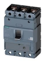
circuit breaker 3VA1 IEC Frame 250 breaking capacity class H Icu=70 kA @ 415 V 3-pole, starter protection TM120M, AM, In=200 A without overload protection short-circuit protection Ii=6...14 x In nut keeper kit
