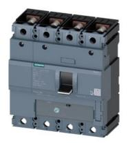
circuit breaker 3VA1 IEC Frame 250 breaking capacity class M Icu=55 kA @ 415 V 4-pole, line protection TM220, ATFM, In=200 A overload protection Ir=140 A...200 A short-circuit protection Ii=10 x In neutral conductor protection 100% nut keeper kit
