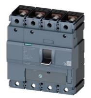
circuit breaker 3VA1 IEC Frame 250 breaking capacity class S Icu=36 kA @ 415 V 4-pole, line protection TM220, ATFM, In=200 A overload protection Ir=140 A...200 A short-circuit protection Ii=10 x In neutral conductor protection 100% nut keeper kit
