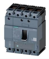
circuit breaker 3VA1 IEC Frame 160 breaking capacity class H Icu=70 kA @ 415 V 4-pole, line protection TM220, ATFM, In=63 A overload protection Ir=44 A...63 A short-circuit protection Ii=10 x In neutral conductor protection 100% nut keeper kit
