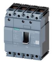
switch disconnector 3VA1 IEC frame 160 4-pole SD100, In=63A without overload protection w/o short-circuit protection nut keeper kit
