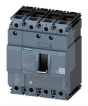
circuit breaker 3VA1 IEC Frame 160 breaking capacity class S Icu=36 kA @ 415 V 4-pole, line protection TM220, ATFM, In=50 A overload protection Ir=35 A...50 A short-circuit protection Ii=10 x In neutral conductor protection 100% nut keeper kit
