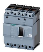
switch disconnector 3VA1 IEC frame 160 4-pole SD100, In=100A without overload protection w/o short-circuit protection nut keeper kit
