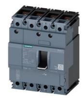
circuit breaker 3VA1 IEC Frame 100 breaking capacity class B Icu=16 kA @ 415 V 4-pole, line protection TM210, FTFM, In=16 A overload protection Ir=16 A permanently set short-circuit protection Ii=20 x In N conductor unprotected nut keeper kit
