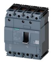
circuit breaker 3VA1 IEC Frame 100 breaking capacity class N Icu=25 kA @ 415 V 4-pole, line protection TM210, FTFM, ln=25 A overload protection lr=25 A permanently set short-circuit protection li=12.8 x In N conductor unprotected nut keeper kit
