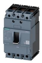
circuit breaker 3VA1 IEC Frame 100 breaking capacity class N Icu=25 kA @ 415 V 3-pole, line protection TM210, FTFM, In=25 A overload protection Ir=25 A permanently set short-circuit protection Ii=12.8 x In nut keeper kit
